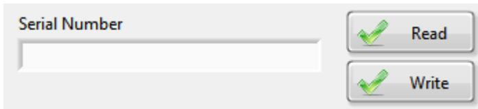
The board serial number can be read here. It is not write protected, and after a warning, it can be changed.
