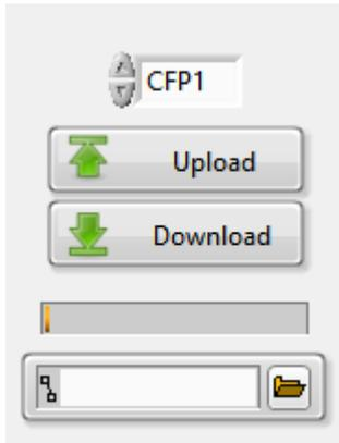
Use the Upload button to load a data file into the CFP. A dialog box will open, where the file to be uploaded is specified.
