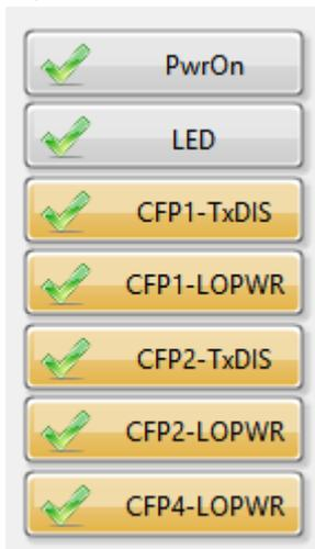
PwrOn controls the power to the CFPs. LED controls the LED to the right of the CFP4 transceiver. The other buttons control the status of various CFP hardware control lines.
